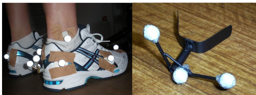
Fig. 1. Image of the markers on the shoe and the device to measure the in-shoe motion of the calcaneus: an array of three markers mounted onto a rigid shaft that attached to the calcaneus via a flexible metal stirrup.
